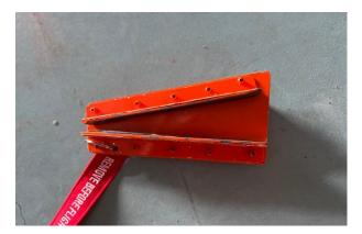
Four pieces of angle pop rivetted to a piece of flat. A small amount of non-slip rubber glued onto angle to prevent scratches and make it a firm fit. Very simple to manufacture
