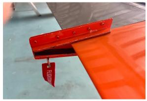
Slide it between the aileron and wingtip
