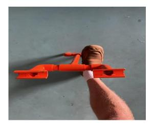
Ends cut to fit over round tubing at bottom of rudder pedals
