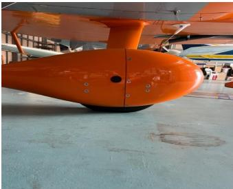
Tyre inflation access point. Sick and tired of removing wheels spats to check tyre inflation? Go to Repco and buy the biggest rubber grommet on the shelf. Drill a hole for access to valve stem, remove valve cap with socket on extension and inflate the tyre. I check my tyres every three months and always have need to put about 6 psi in every time, tubes do not hold pressure forever
