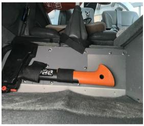
Velcro tape raps around my emergency exit (light weight) axe (Fiskars brand). Axe is also good for hammering ground stakes in and smashing canopy open in emergency. In my case I secure the Velcro around the axe handle and this holds the rudder gust lock down and firm.
