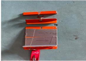
The top two angle pieces are removable and are secured by one machine screw and wing nut.
