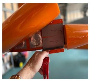
Slide or place the flat plate between the elevator and horizontal stabliser
