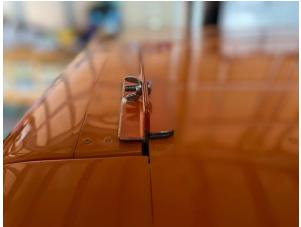
Lock the two top pieces of angle together and the gust lock is secure
