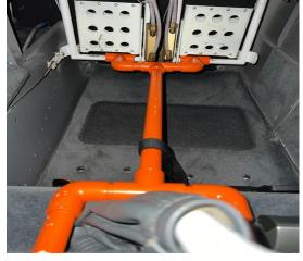
Install over rudder pedals and lock back onto vertical shelf associated with control stick. Note Velcro tape holding lock down and secure, otherwise conduit can walk upwards and free itself in gusty conditions
