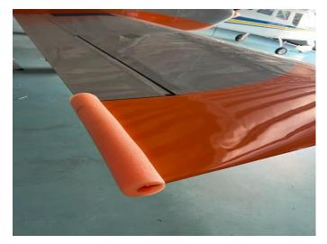
Hangar Rash: Pool Noodle fitted to wing tip, prevents wing tip damage when someone else moves your plane around in the hangar. Guess how I worked this one out?
